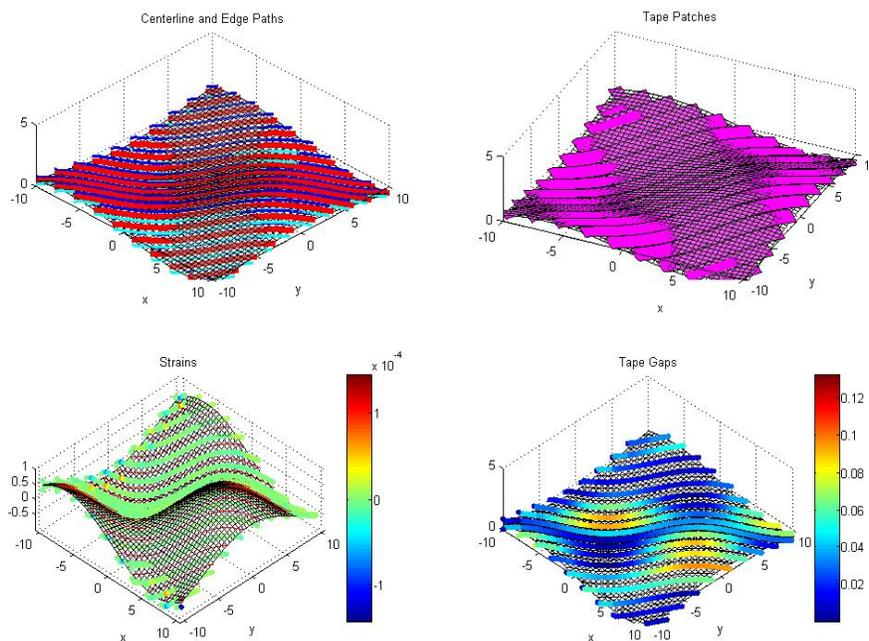
Figure 1. Tow trajectories, patches, strains and gaps for ATL model of a sinusoidal surface.
