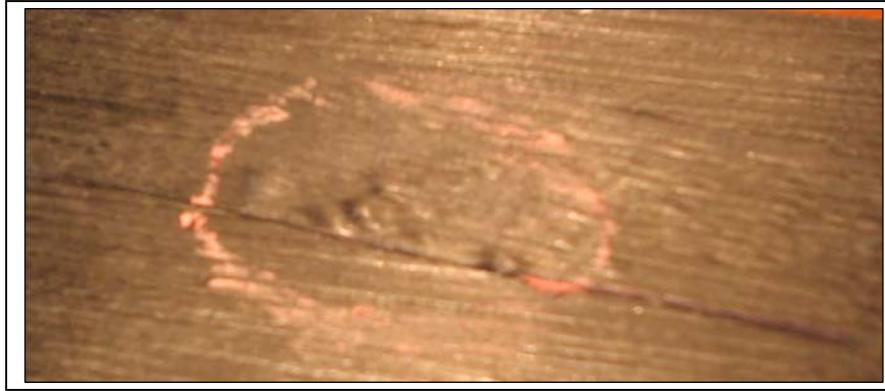
Figure 2. Macro buckling of a 13mm tow aligned along a radial path of 900 mm.
