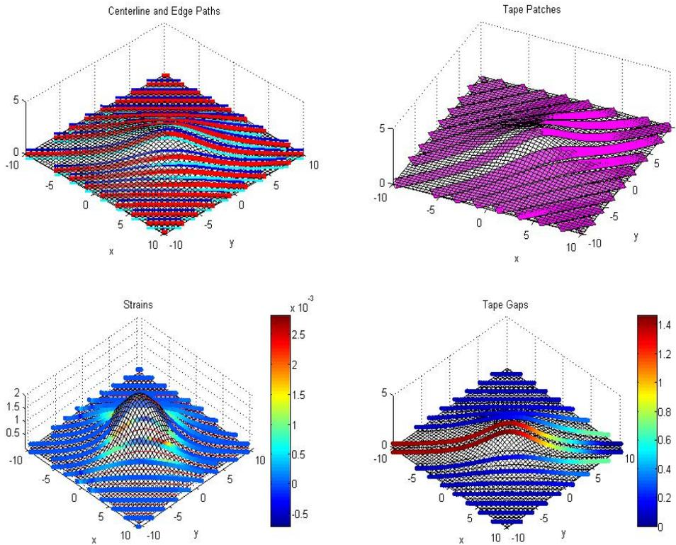
Figure 6. Natural paths over single hump geometry with constant initial angle of 45deg.
