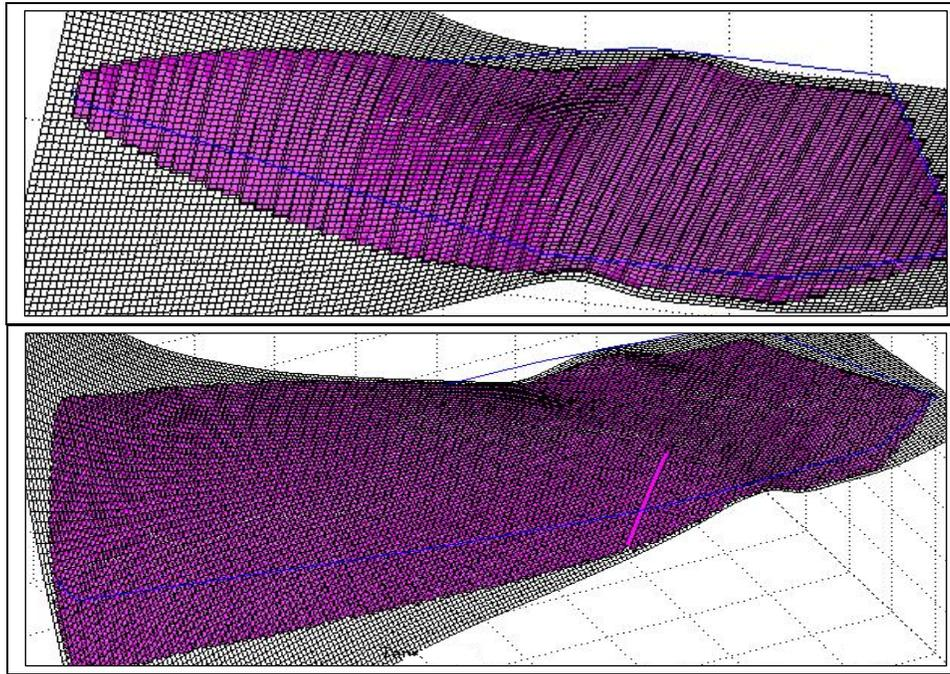
Figure 11. Top: Ninety degree rotor blade ply with 13mm tow. Lower: Forty five degree ply with 7mm tows.
