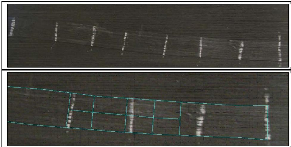
Figure 3. Image processing used to calculate strains of tows along curved trajectory.
