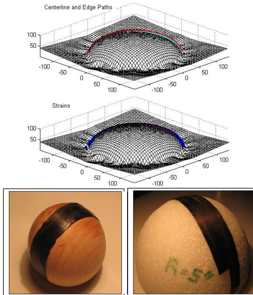
Figure 4. Computational (top) and experimental wrapping (bottom) of tows around spherical surfaces with constant curvature.
