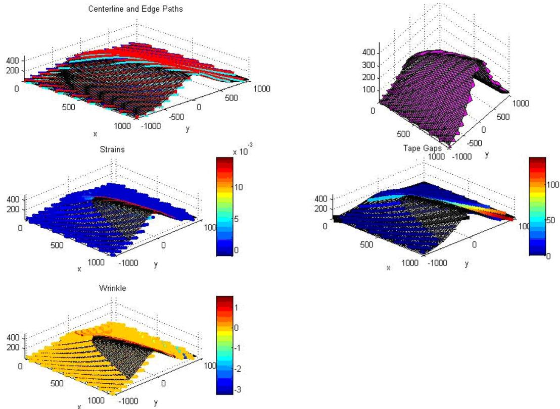
Figure 10. ATL simulated covering of aircraft cowling.
