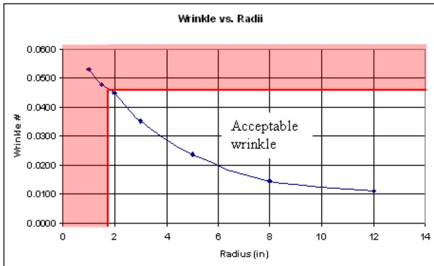
Figure 5. Computational wrinkle values corresponding to a give surface radius. Problem wrinkles occur at a wrinkle value greater than 0.0475.
