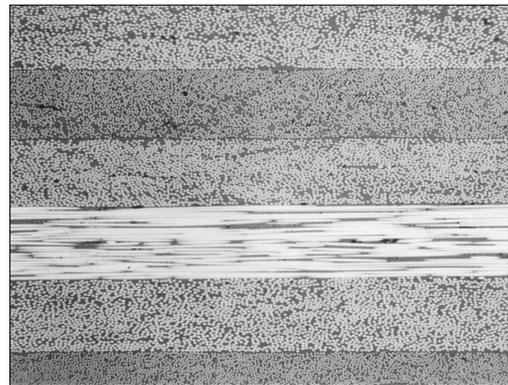
Figure 1.2 Photomicrograph of high quality IM-7/PIXA laminate from TP-ATP and placement-grade tape
