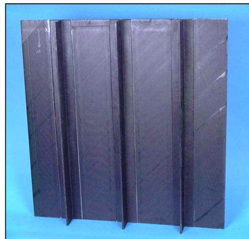
Figure 1.4 In situ placed three-stringer laminate
