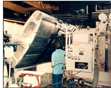
*Figure 4.2-1 The ATP head has a single process spot to fabricate laminates with complex geometry*
