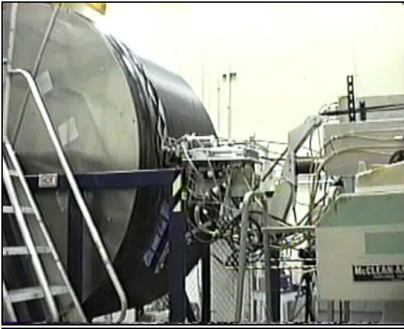
Figure 2.1 Heated filament winding head for hoop (90°) plies
