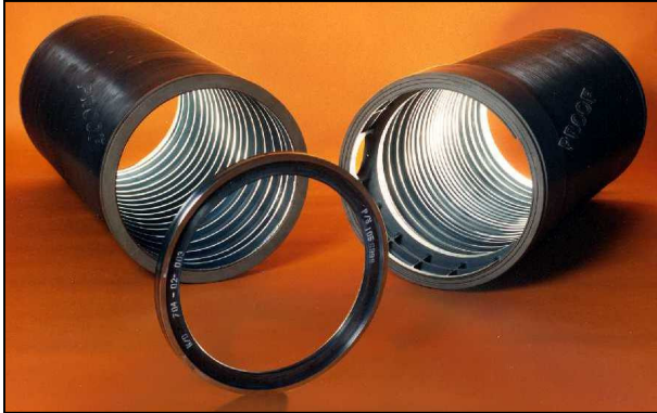
Figure 3.4 Filament wound/tape laid APC-2/IM-7 [90^\circ/0^\circ]_n and [90^\circ_2/0^\circ]_n ring-stiffened underwater vehicle hull sections
