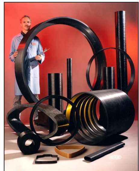
Figure 4.1 Carbon and glass thermoplastic filament-wound cylinders up to 152cm (60-in).
