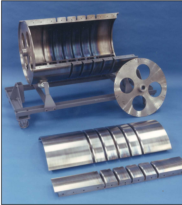
Figure 3.1 Innovative collapsible tooling is used to wind ring-stiffened cylinders
