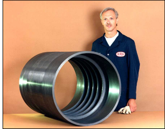
Figure 3.2 61cm diameter 16mm thick ring-stiffened APC-2/AS-4 cylinder
