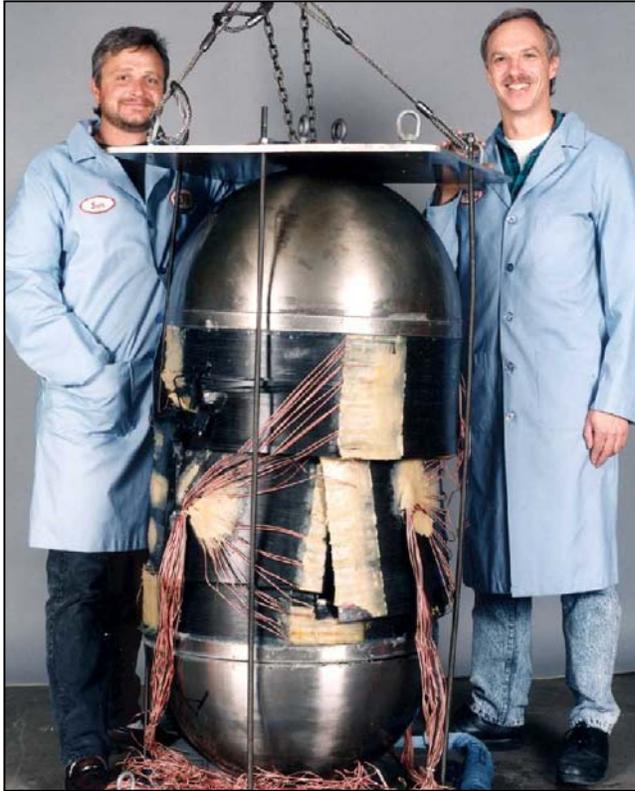
Figure 4.1 In the test, the cylinder failed at 37.9 MPa (5500 psi), within 3% of prediction.
