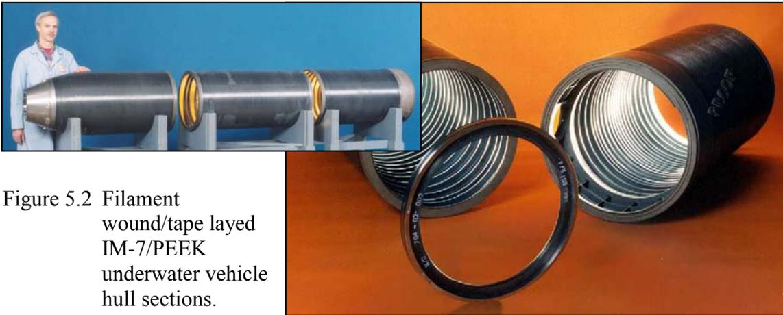
Figure 5.2 Filament wound/tape layered IM-7/PEEK underwater vehicle hull sections.
