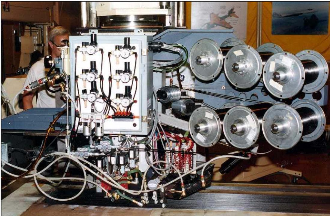
Figure 6.2 Deposition head in situ consolidating 12 thermoplastic tows.
