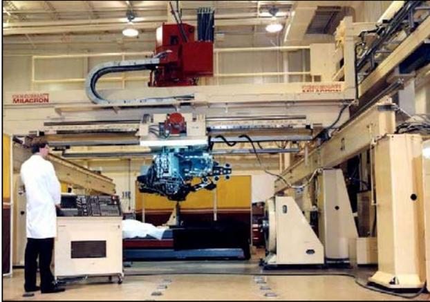
When equipped with a tow feeder, the head is a "TCA" or Tow Cut and Add head and additionally allows variable deposition of tows for steering or placement on contoured geometry. The tow feeder uses a 12-position creel, and has a capacity of 54kg (120lb). The tow feeder can be replaced with the 76mm (3-in) tape feeder. Changeover from tow to tape mode takes about two hours.
