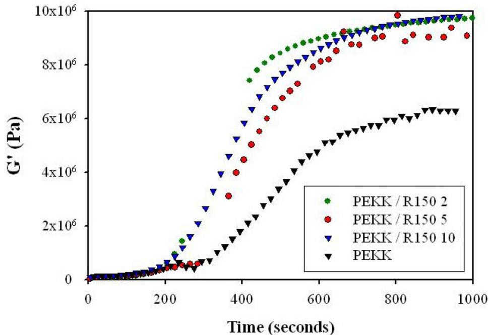
Figure 8. Development of elastic moduli during crystallization annealing time at 238°C of the PEKK / Aerosil R150 blends as monitored through parallel plate rheological experiments.
