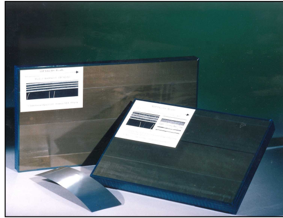
Figure 9.2 TiGr honeycomb laminates made by interleaving titanium and IM-6/PEEK plies using the primary bonded honeycomb process.
