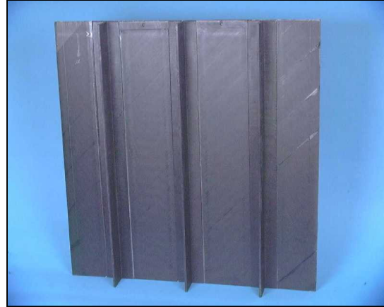
Figure 7.2 Placing the first few courses of a stringer-stiffened panel over embedded pre-cured thermoplastic stiffeners, and finished three-stringer panel.
