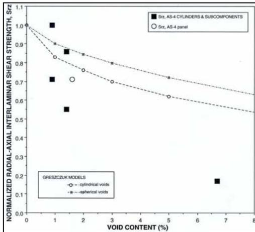
Figure 2.3 Void content negatively affects interlaminar shear strength
