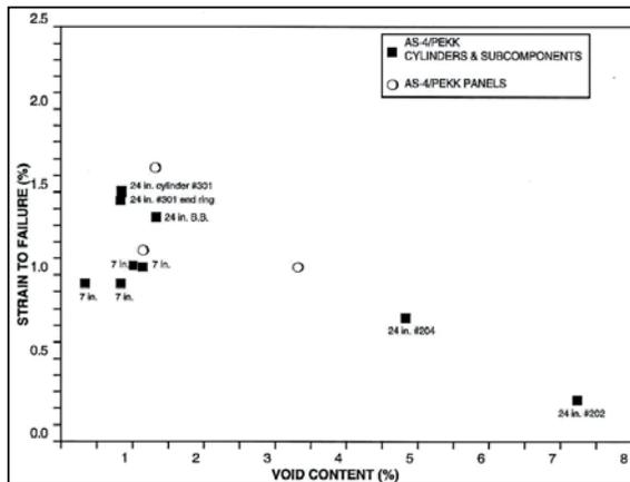
Figure 2.2 Compression Strain-to-Failure for AS-4/PEKK Cylinders and Laminates
