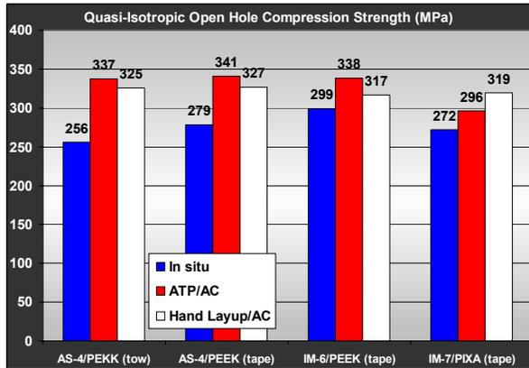
Figure 3.2 OHC for PEKK, PEEK & PIXA
