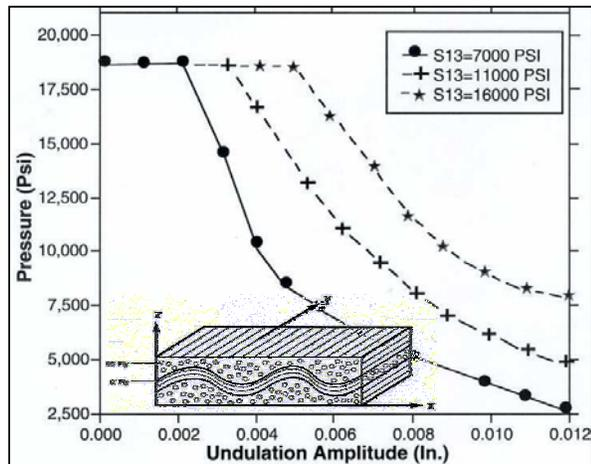
Figure 2.4 Influence of waviness undulation amplitude on collapse pressure of AS-4/carbon PEEK and PEKK cylinders
