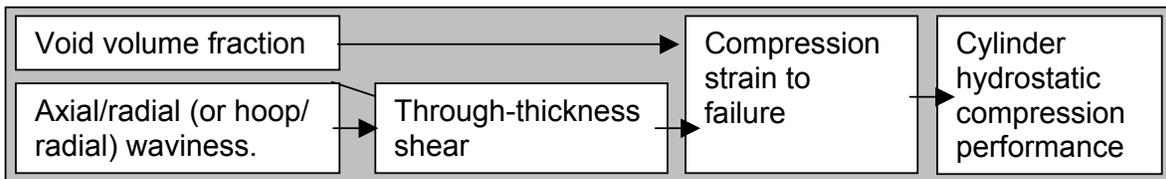
Figure 2.1 The effect of void content and waviness, through shear, on compression strain-to-failure and then to cylinder hydrostatic compression load carrying capability
