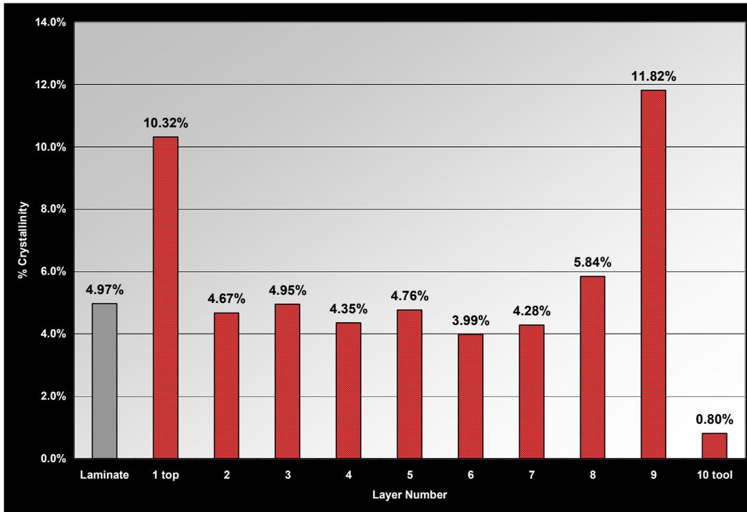
Figure 3.4 Crystallinity through the thickness for an AS-4/PEKK laminate processed on an unheated insulated composite tool.
