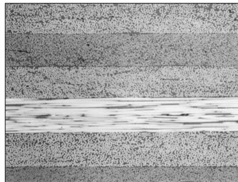
Figure 3.1 A quasi-isotropic laminate fabricated from IM-7/PIXA tape with an in situ consolidation tape placement process is void and waviness free
