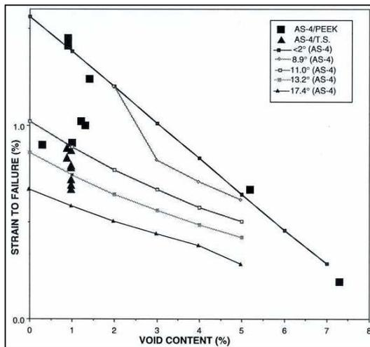
Figure 2.5 combines the synergistic effect of voids and waviness on strain-to-failure. Voids alone reduce compression strain-to-failure in cylinders with waviness less than 2°. Increasing void content acts to reduce shear strength, and through waviness, also lowers the compression strain-to-failure even further than voids alone.
