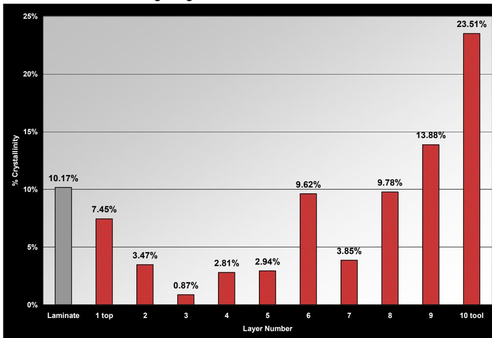
Figure 3.3 Crystallinity through the thickness for an AS-4/PEKK laminate processed on an aluminum tool heated to 175°C. Maximum PEKK crystallinity is 26% to 29%.
