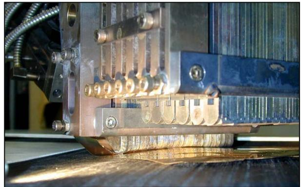
Figure 16 The shim was removed to show the shim conformance against the laminate from the back side.
