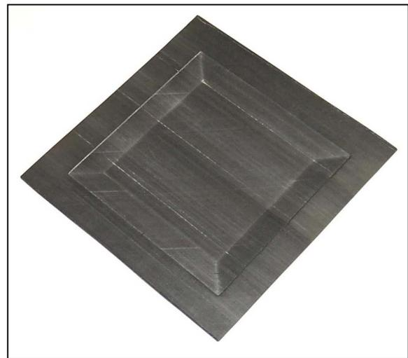
Figure 13 Tool surface of [0/-45/90/45]<sub>2s</sub> pad-up laminate produced on pyramid shaped tool
