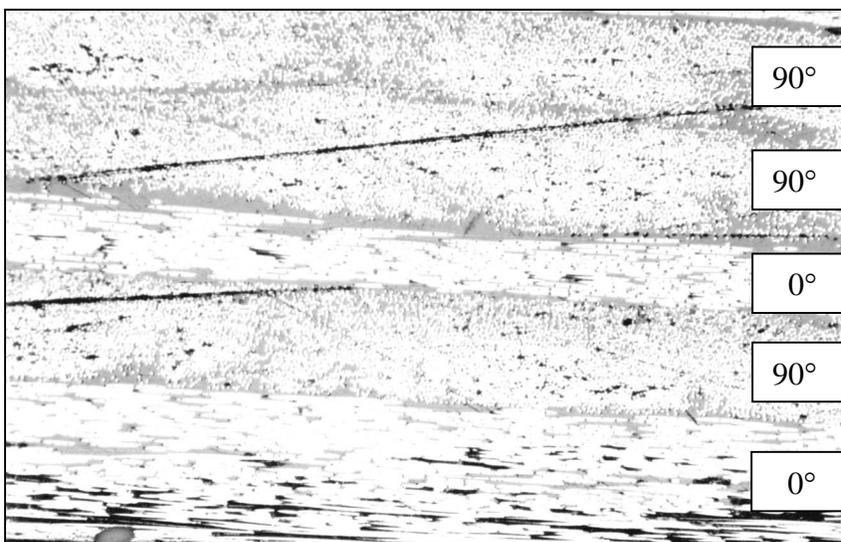
There are no apparent voids at the interface between the  $0^\circ$  and  $90^\circ$  plies, and between the  $90^\circ$  and  $90^\circ$  plies. Some dark spots exist at the bottom  $0^\circ$  ply due to polishing. Note also the void reduction that has taken place in the IM-7/PEEK tape. There are few interlayer voids left.
