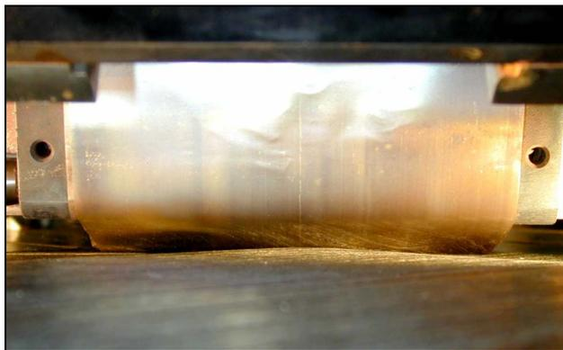
Figure 15 The head is placing in a 45° course direction over the center of the laminate, where two ramps come together to form a crease.
