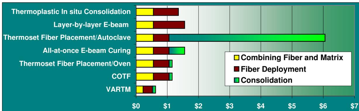
Figure 2 Comparison of the cost of material and equipment acquisition amortized for ten Reusable Launch Vehicle LH<sub>2</sub> tanks (millions of dollars)
