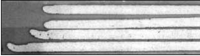
Figure 4 Photomicrograph cross-section showing four very nice quality thermoplastic ribbons
