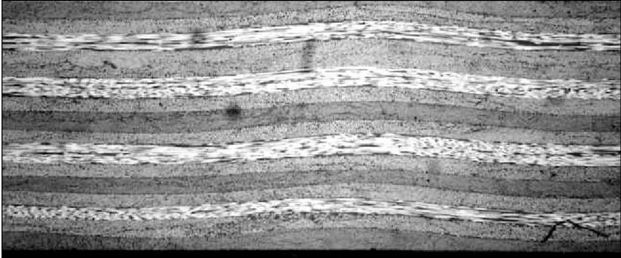
Figure 7 Photomicrograph of laminate with two tows placed directly over one another in the base ply. The ply undulation is reproduced throughout the laminate thickness.
