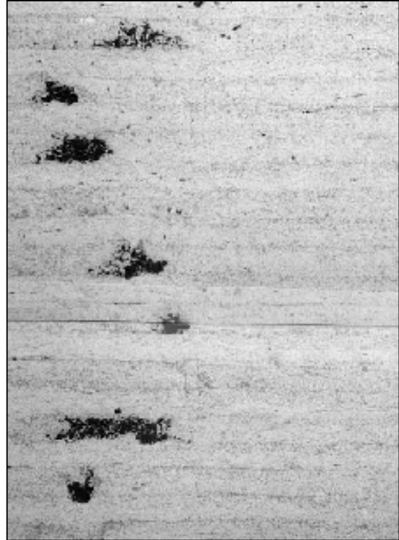
Figure 6 shows a laminate fabricated over a missing thermoplastic ribbon. The layers placed on top could not fill the space left. This shows what happens when a rigid compactor is employed and there are thickness variations in the incoming ribbons or tapes, or there is a tape overlap or ply add. A rigid compactor concentrates force on high spots, but low spots are not substantially compacted, leading to a significant loss of quality.
