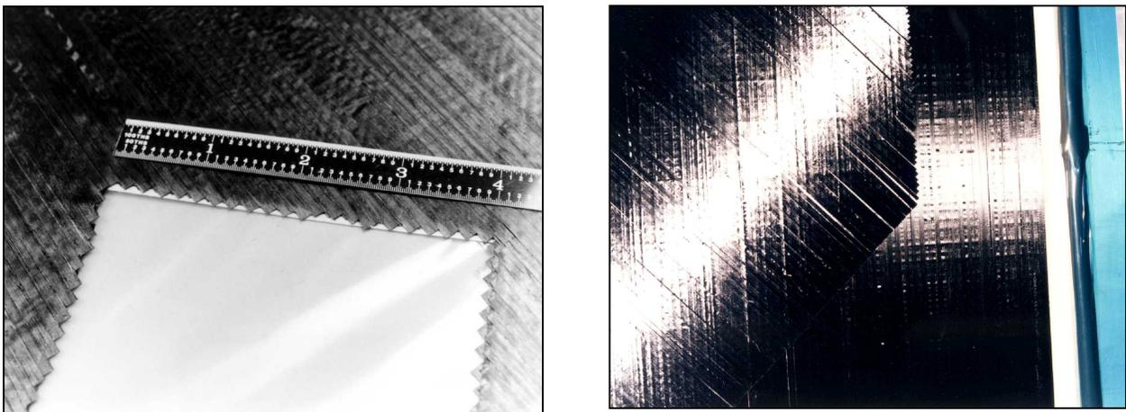
Figure 8 Tow cut and adds around cut outs and ply adds requires  $\pm 760\mu\text{m}$  ( $\pm 30\text{-mil}$ ) accuracy on ends, requiring slow placement velocity.
