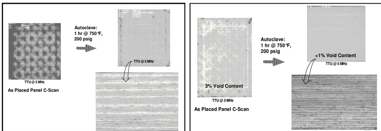
Figure 3 Ultrasonic C-scan and photomicrographs of thermoplastic in situ consolidated laminates made via placing three-inch tape. The autoclave consolidation process significantly improved the laminate.
