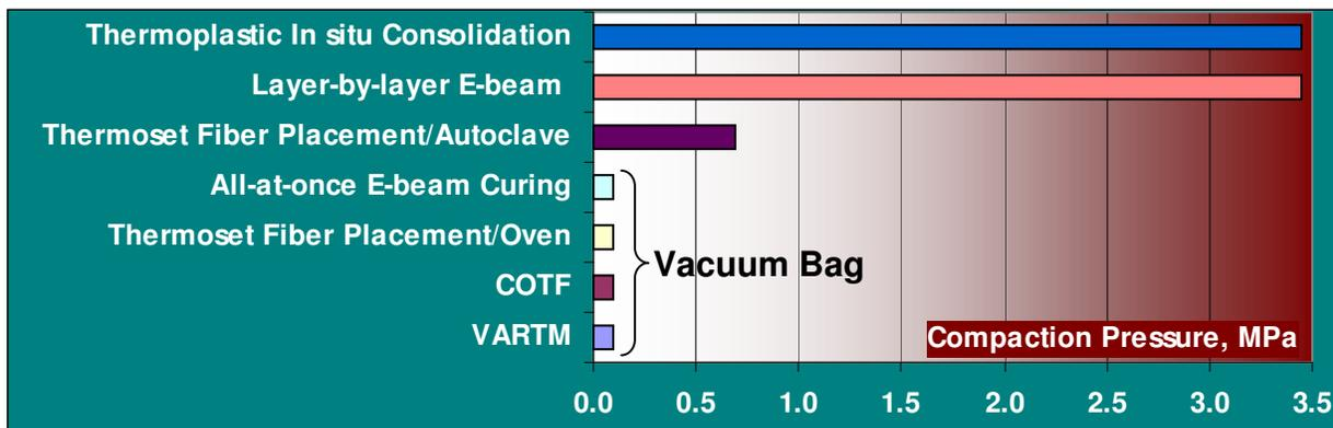
Figure 1 Four processes provide only provide vacuum bag pressure, but thermoset fiber placement/autoclave curing, layer-by-layer E-Beam, and thermoplastic in situ consolidation can provide as much as 3.4 MPa (500 psi) compaction pressure.
